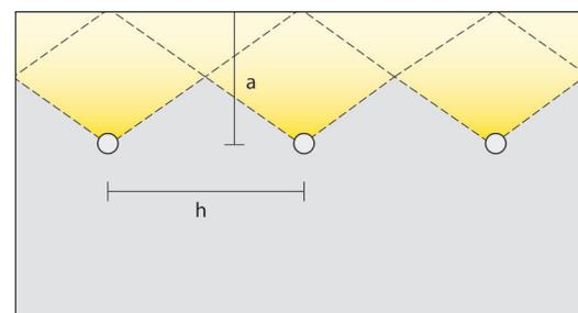
In order to have uniform lighting, it is best that the distance between two light fixtures are 1/3 of room height. Valman fixtures are a perfect solution for walls up to 6 meters
