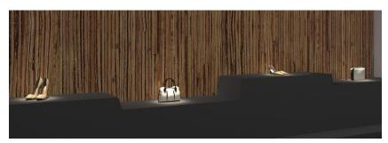
The ceiling height in your shop is almost 5 meters and you have a small object which you want to highlight? That's very easy with Nian XS. Due to extremely narrow beam light, a circle with diameter of only 65 cm illuminated even from a distance of 4 meters between the light source and show case.
